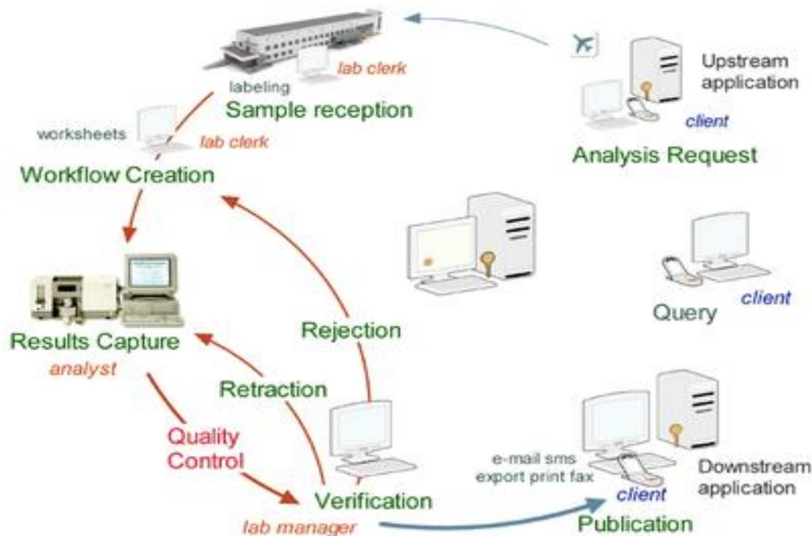
Figure 2. A schematic illustration of a typical LIMS integrated into the sample receipt, analysis and generation of certificates of analysis for the client. [9].
